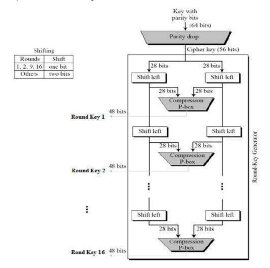
The logic for Parity drop, shifting, and Compression P-box is given in the DES description.
