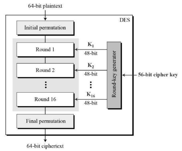
Since DES is based on the Feistel Cipher, all that is required to specify DES is -
