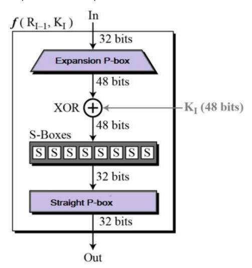
• **Expansion Permutation Box** — Since right input is 32-bit and round key is a 48-bit, we first need to expand right input to 48 bits. Permutation logic is graphically depicted in the
