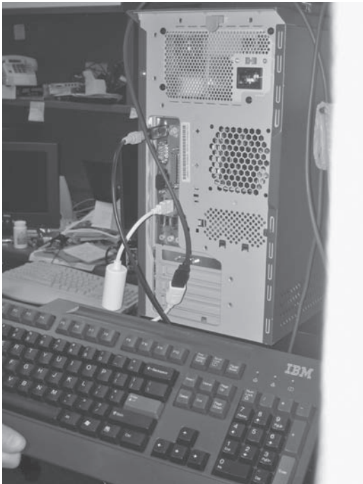
Keyloggers are mechanisms which capture information from installed keylogging devices. Software keyloggers also provide screenshot features, which users can utilize to view screenshot images of victim activity. Hardware and software keyloggers have varying advantages and disadvantages. Hardware keyloggers can be easily installed and removed. The photo contains two such devices. One is plugged into the USB port and the other connects the keyboard to the CPU. Both devices were generously donated by KeyGhost. (Dr. Marjie T. Britz, Ph.D.)
