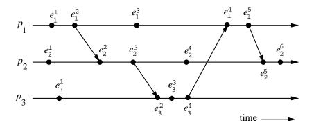
Figure 2.1: The space-time diagram of a distributed execution.
