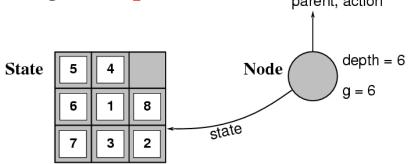
The Expand function creates new nodes, filling in the various fields and using the SuccessorFn of the problem to create the corresponding states.
